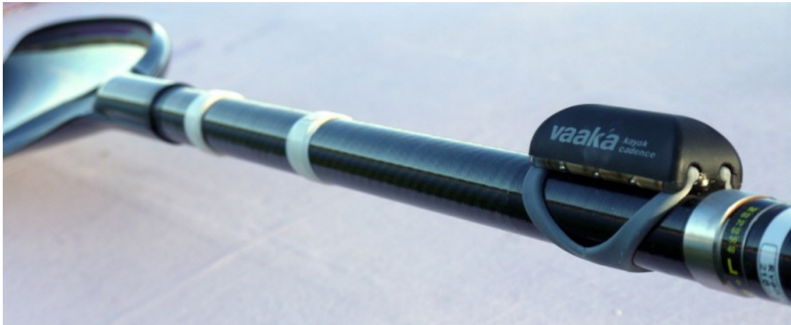
Fig. 2. Cadence sensor attached to kayak paddle ready for calculating and transmitting cadence information to a compatible device.
